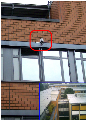
Fig. 10. Quadrotor (red square) flying near the building. It can carry a camera which allows us to acquire an interior overview through windows. Lower right (blue square) shows the camera view of the quadrotor flying above roofs.
