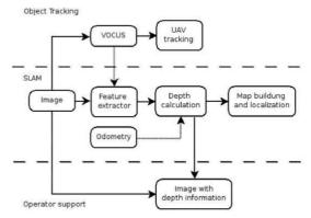
Fig. 10: SC<u>HEMATIC OVERVIEW OF THE VISION S</u>YSTEMS. <sup>3</sup> http://de.youtube.com/watch?v=LKmCPMNUYZs
