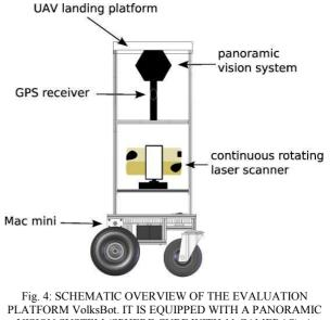
PLATFORM VolksBot. IT IS EQUIPPED WITH A PANORAMIC VISION SYSTEM (SPHERE CUBE WITH 11 CAMERAS), A CONTINUOUS ROTATING 3D LASER SCANNER, A GPS RECEIVER, A LANDING PLATFORM FOR THE QUADROTOR, BATTERIES AND CONTROL COMPUTERS.
