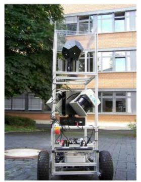
Fig. 1: FIRST EVALUATION PLATFORM OF THE UGAV. THE GROUND PLATFORM IS BUILD OF A VOLKSBOT RT3 WHICH IS EQUIPPED WITH BATTERIES, VISION SENSORS, 3D LASER SCANNER, CONTROL COMPUTERS AND A LANDING PLATFORM ON TOP FOR THE QUADROTOR.
