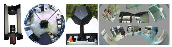
Fig. 2 VISIONS SYSTEMS FOR THE UGV. (A) SHOWS THE OMNIDIRECTIONAL IAIS VISION SYSTEM. THE CAMERA AIMS TOWARDS A HYPERBOLIC MIRROR. (B) IS AN IMAGE FROM THE PERSPECTIVE OF THE OMNIDIRECTIONAL CAMERA. (C) THE DODECAHEDRON SHAPED CAMERA SYSTEM WITH ELEVEN CAMERAS. EACH CAMERA AIMS IN ANOTHER DIRECTION. (D) DEMONSTRATES AN IMPRESSION FROM PANORAMIC IMAGES OF THE DODECAHEDRON.
