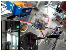
Fig. 14: A PROTOTYPE OF THE QUADROTOR USED FOR THE EVALUATION. ON THE BOTTOM-LEFT FIGURE THE COPTER IS TESTED FOR LANDING ON A SMALL PLATFORM IN THE FRAUNHOFER IAIS ROBOTIC LABORATORY.
