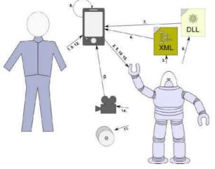
Fig. 7: OCU AND ROBOT INTERACTION OVERVIEW. 1: AN OPERATOR SELECTS THE ROBOT ON THE MOBILE DEVICE, 2: OCU-SOFTWARE CONNECTS TO ROBOT AND REQUESTS THE RKI-FILE, 3-4: ROBOT SENDS DESCRIPTION, 5: OCU-SOFTWARE REQUESTS CONTROL PLUGINS, 6-8: ROBOT SENDS PLUGINS, AND OCU ADAPTS ITS SELF, 9-10: OPERATOR SELECTS AN ACTION FOR THE ROBOT (E.G. MOVE) AND THE OCU TRANSMITS THE NEEDED COMMANDS, 11: ROBOT RECEIVES AND EXECUTES COMMAND, 12-13: OPERATOR DEMANDS SENSOR DATA, 14-15: ROBOT SENDS THE SENSOR DATA...
