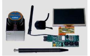
Fig. 13: FROM THE LEFT TO THE RIGHT A HOKUYO URG-04LX LASER RANGE-FINDER, A WIRELESS VISORTECH GP-811T CAMERA AND GUMSTIX VERDEX XL6P COMPUTER WITH 802.11 (G) WIRELESS COMMUNICATION MODULE ARE SHOWN. THE DISPLAY IS DETACHABLE AND IS NOT NEEDED DURING THE FLIGHT.
