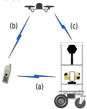
Fig. 6: UNMANNED GROUND-AIR VEHICLE (UGAV): THE MOBILE DEVICE CONTROLS EITHER THE UGV (A) OR THE UAV (B). (C) UAV IS COMMANDED BY THE UGV.
