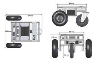
Fig. 3: ENGINEERING DRAWING OF THE VolksBot RT3 CHASSIS. RT3 IS A THREE-WHEELED ROBOT PLATFORM. THE LEFT SKETCH SHOWS TOP VIEW, UPPER RIGHT SHOWS LATERAL VIEW AND LOWER RIGHT SHOWS FRONT VIEW.
